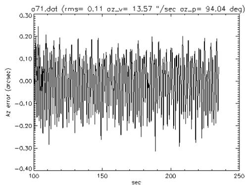
Fig.1 - Azimuth Error (Speed = 13 arcsec/sec)
