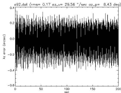
Fig.2 - Azimuth Error (Speed = 30 arcsec/sec)
